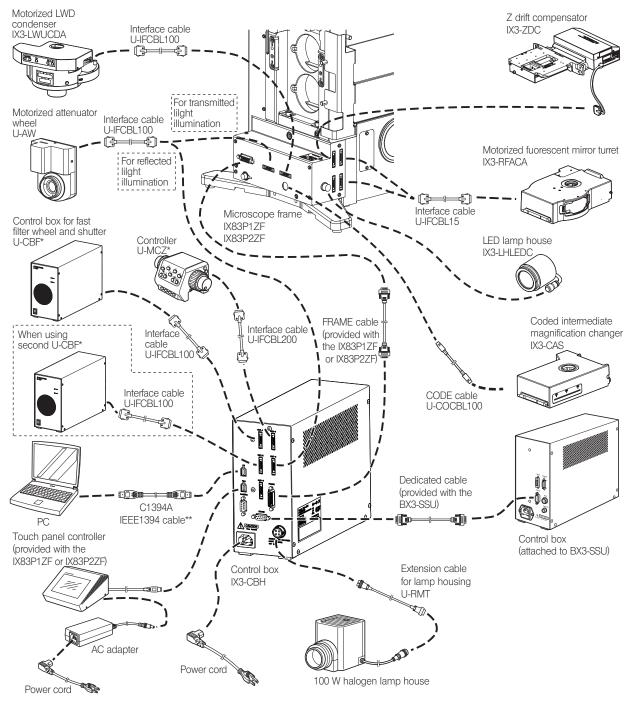
\* The OUT 1 to 5 connectors accept the connections of the U-AW, U-MCZ, etc.
