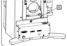
Releasing the transport lock of the focusing mechanism
