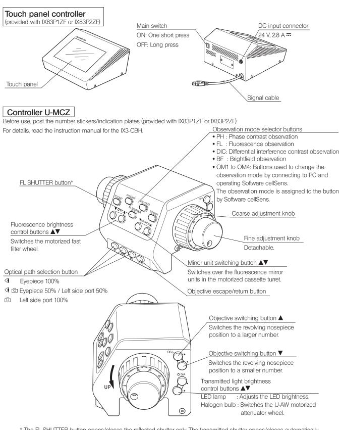
\* The FL SHUTTER button opens/closes the reflected shutter only. The transmitted shutter opens/closes automatically depending on the observation modes.
