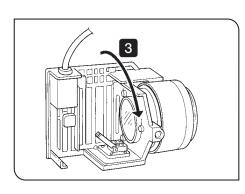
4 While pushing down the bulb clamping lever a, hold the halogen bulb b with gloves or a piece of gauze, insert the bulb pins c straight and fully into the pin position d on the lamp socket. Then return the lamp clamping lever gently back to the original position to clamp the bulb.
