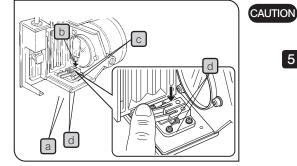
To prevent reduced bulb life or cracking, do not touch the bulb with bare hands. If fingerprints are accidentally left on the bulb, wipe the bulb with a dry soft cloth.
