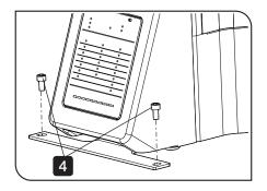
**4** Tighten the fixing screw by using the commercially available 5 mm Allen wrench to secure the microscope on the anti-vibration table.
