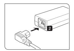
2 Insert the connector of the power cord firmly into the input connector of the AC adapter.
