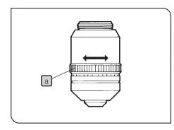
If the thickness of the cover glass or the vessel does not match the thickness scale of an objective with correction collar, the objective cannot manifest its performance. When using a correction collar equipped objective, perform the following adjustment as required.
