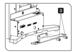
3 Attach the fixing plate on the back side of the microscope and fix it by using the commercially available 5 mm Allen wrench.
