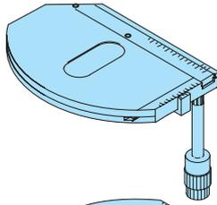
Specimen holder for mechanical stage
