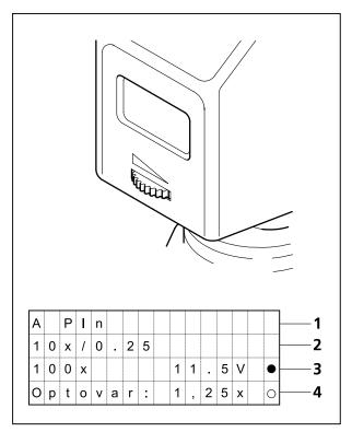
Fig. 4-15 LCD display
