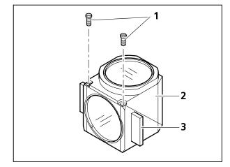
Fig. 3-23 Changing the beam splitter
