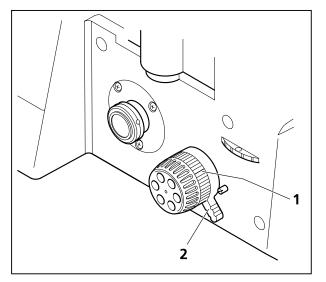
Fig. 4-14Vertical stop for focus drive
