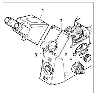
Fig. 3-2 Attaching the binocular tube
