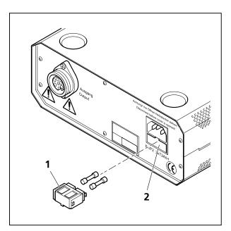
Fig. 5-2 Replacing the power supply fuses
