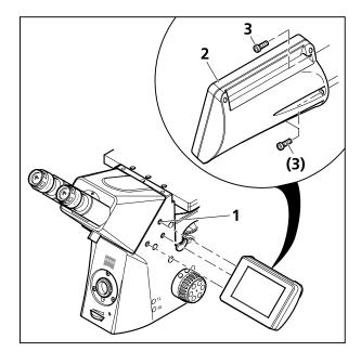
Fig. 3-26 Fitting the TFT display
