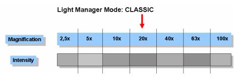
Fig. 4-20 Illumination intensity looking into the eyepieces, changing only the objective (starting from 20x). Light Manager settings for each objective have been saved previously.
