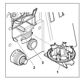
Fig. 3-19 Fitting the reflector turret
