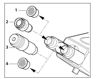
Fig. 3-3 Inserting the eyepieces
