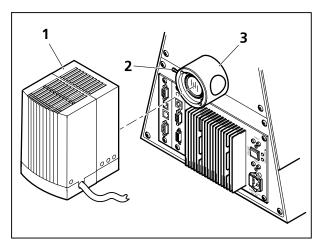
Fig. 3-39 Attaching the HBO 100 illuminator
