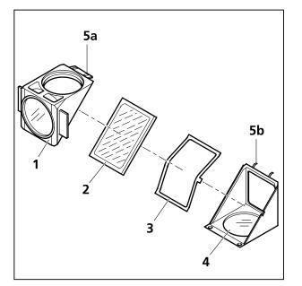
Fig. 3-24 Changing the beam splitter
