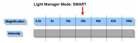
Fig. 4-21 Illumination intensity looking into the eyepieces, changing only the objective (starting from 20x). Settings for one objective have been saved previously.
