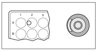
Fig. 4-71 VAREL contrast for microtiter plates
