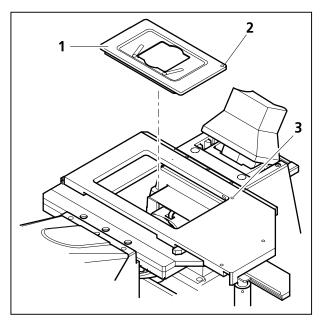
Fig. 3-9 Fitting the mounting frame K
