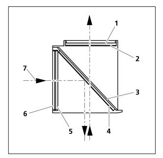
Fig. 3-22 Installing the filter and beam splitter
