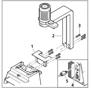
Fig. 3-6 Fitting the 35 W transmitted light illuminator carrier
