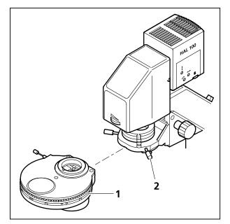
Fig. 3-16 Attaching the condenser
