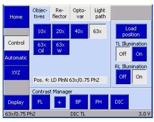
Fig. 4-30 Page Microscope -> Control -> Objectives
