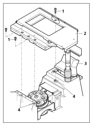
Fig. 3-8 Fitting the mechanical stage 130x85
