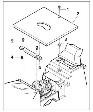
Fig. 3-13 Attaching the specimen stage 250x230
