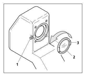
Fig. 3-37 Fitting and removing the diffuser
