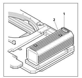
Fig. 3-12 Scanning stage 130x85 mot. CAN, connections on the underside
