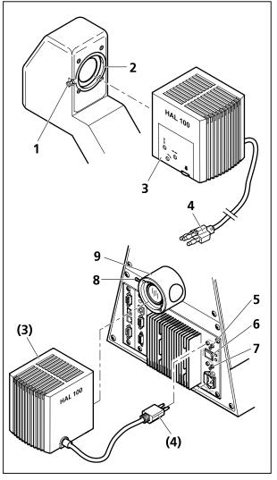
Fig. 3-35 Attaching the HAL 100 halogen illuminator
