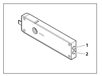
Fig. 4-9 FL attenuator, motorized
