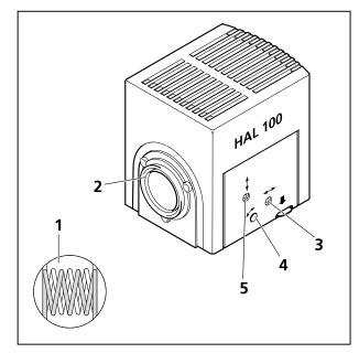
Fig. 3-36 Adjusting the HAL 100 halogen illuminator
