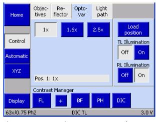
Fig. 4-32 Page Microscope -> Control -> Optovar
