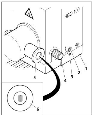
Fig. 3-41 Adjusting the HBO 100
