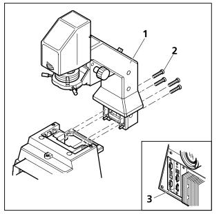
Fig. 3-5 Fitting the 100 W transmitted light illuminator carrier
