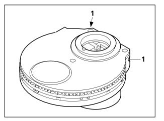
Fig. 4-67 Centering the condenser phase stop
