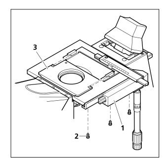
Fig. 3-14 Fitting the object guide and mounting frame
