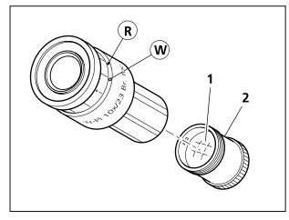
Fig. 3-4 Inserting the eyepiece reticle
