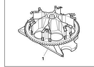
Fig. 4-10 6-position reflector turret
