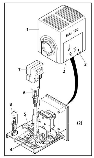
Fig. 3-38 Replacing the halogen bulb
