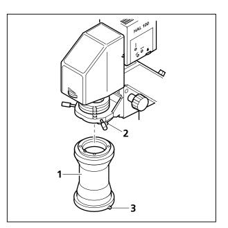
Fig. 3-17 Fitting the condenser carrier
