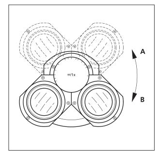
Fig. 4-13 Setting the binocular tube eyepiece distance
