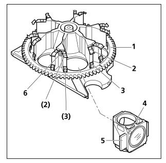
Fig. 3-20 Fitting the reflector modules
