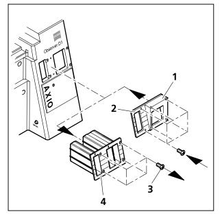
Fig. 3-43 Fitting the Laserport adaptor
