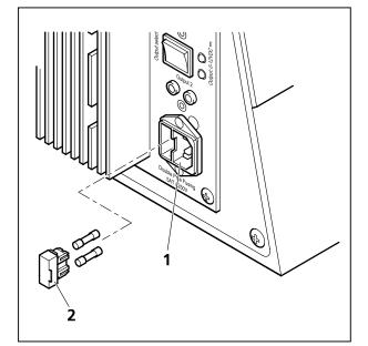
Fig. 5-1 Replacing the fuse
