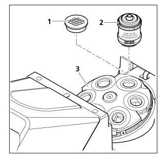
Fig. 3-7 Screwing in the objectives
