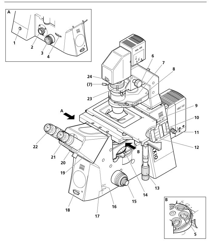
Fig. 4-1 Axio Observer.A1 components and controls (manual)
