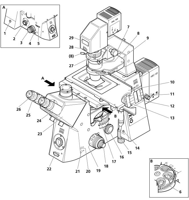
Fig. 4-2 Axio Observer.D1 components and controls (coded, semi-motorized)
