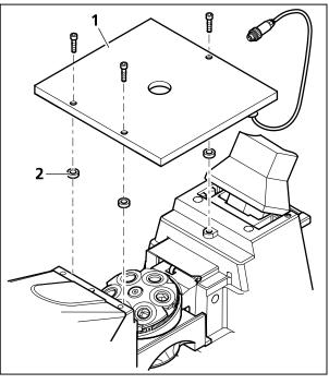
Fig. 3-15 Fitting the heating stage
