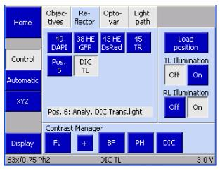
Fig. 4-31 Page Microscope -> Control -> Reflector
